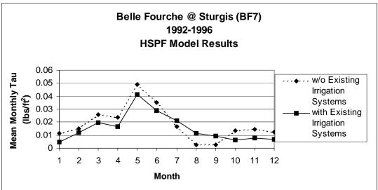
Figure 26. Monthly flow and shear stress, BF7, with and without existing irrigation.
