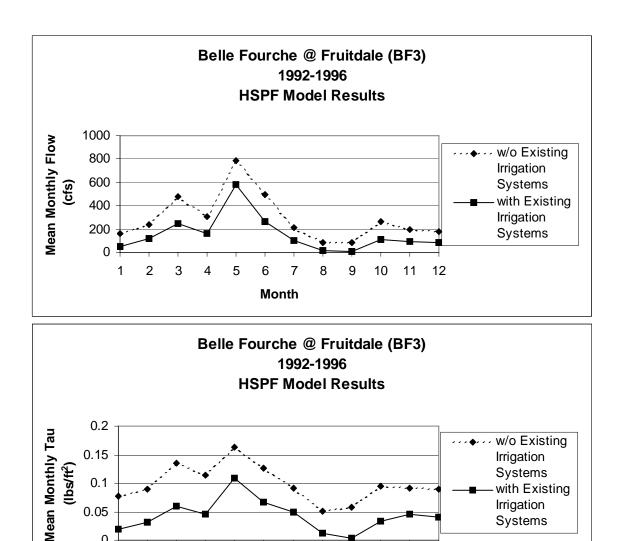
Figure 25. Monthly flow and shear stress, BF3, with and without existing irrigation.
