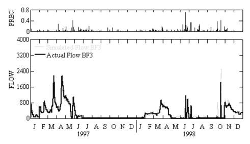
Figure 21. Comparison of simulated and actual flow during validation period at BF3.
