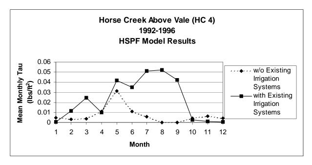
Figure 24. Monthly flow and shear stress, HC4, with and without existing irrigation.
