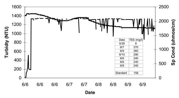
Figure 9. Change in turbidity and specific conductance due to Keyhole Reservoir releases (2002).
