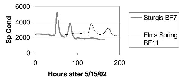
Figure 10. Specific Conductance response to BFID canal/laterals startup.
