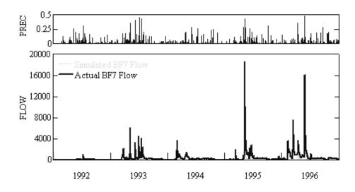
Figure 16. Comparison of simulated and actual flow at BF7.
