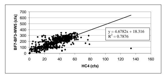
Figure 14. Regression to determine additional flows from BFID as a function HC4 (Irrigation season 1992-1996 without storm flows).
